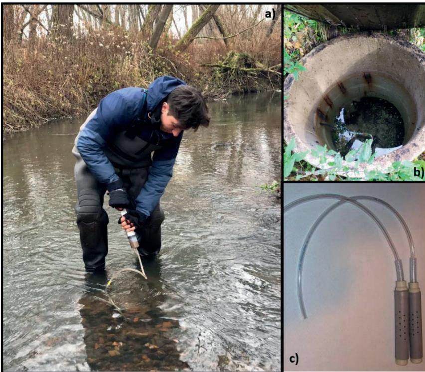
*Figure 12.* a) Sampling procedure for extracting hyporheic water from nests, b) typical domestic well sampled during this study, and c) hyporheic water sampler installed in the nests to withdraw the water (Manuscript III, in preparation).
